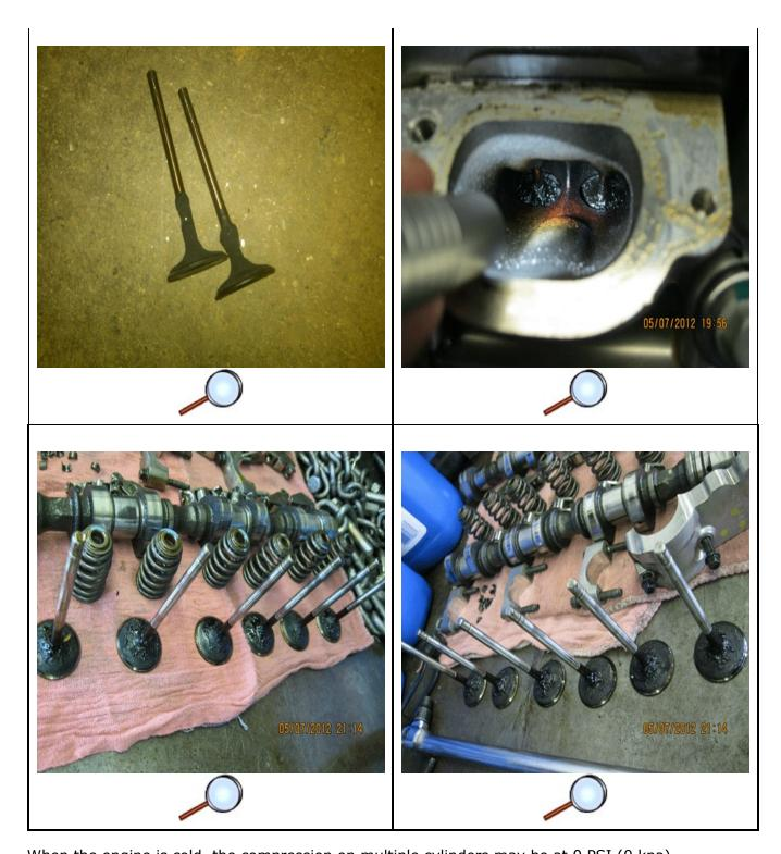
When the engine is cold, the compression on multiple cylinders may be at 0 PSI (0 kpa).
