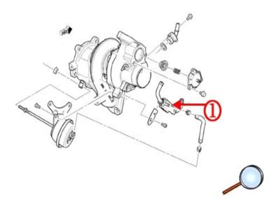
This solenoid is available separate from the turbocharger and should be replaced as a sub assembly. Do not replace the turbocharger assembly.
