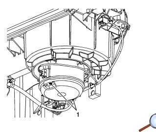
2. Remove the lower blower motor cover heat stakes (1) with a small chisel.
