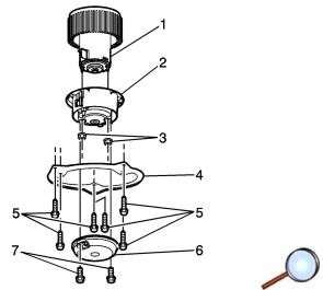
1. Install the blower motor (1) into the motor cup (2) that was cut out of the lower case.
