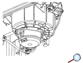
7. Connect the blower motor electrical connector.
