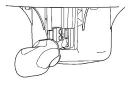
6. Release the blower motor retaining tab and remove the motor from the cup.
