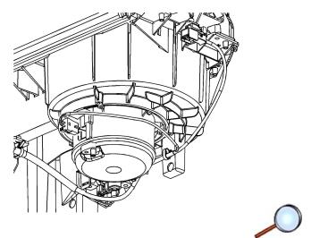
1. Disconnect the blower motor electrical connector.
