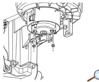
4. Remove the blower motor nuts.
