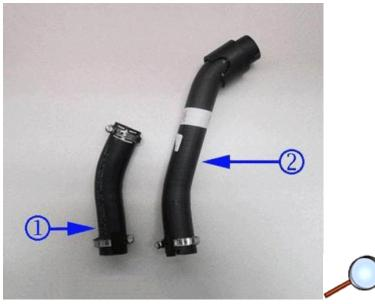
3.2. Match the new hose (2) to the original (1), aligning side by side.
