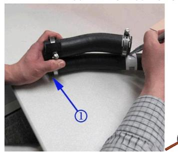
3. Using a paint pen or equivalent, mark the new hose to the original, starting with the notched fuel tank ends of the hoses so that both hoses are the same length.
