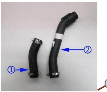
2. Match the new hose (2) to the original (1), aligning side by side.
