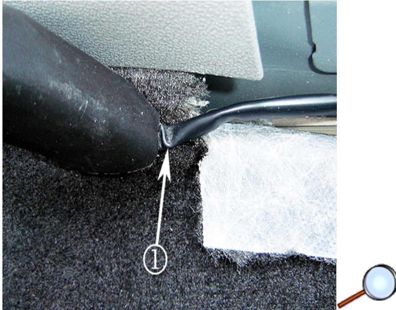
Figure 2 - Outer Wiring Wrap Insulation Breached
